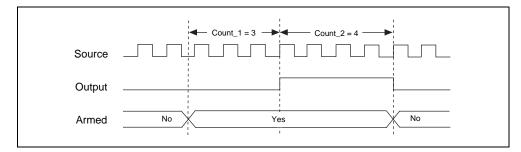
Figure 2-19. Single Pulse Generation
